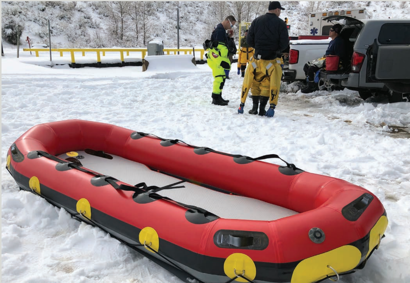
Removable laced-on sacrificial bottom option shown above mitigates damage and abrasion when traversing rugged surfaces.
