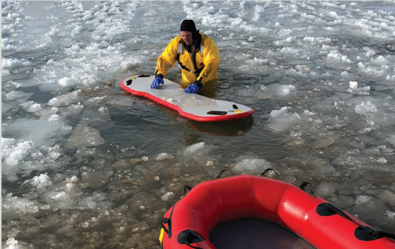
Removable / throwable floor can be used to stabilize a victim while additional rescue tools are deployed.
